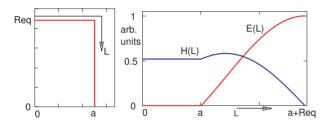
Figure 6: Fields on the surface of a pillbox cavity.
