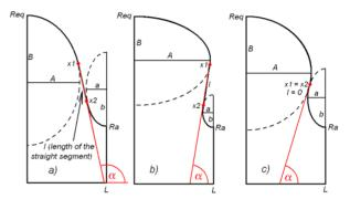
Figure 1: Geometry of the elliptic half-cell: non-reentrant -a), and reentrant -b) and c).
