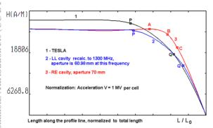
Figure 3: Surface electric field of the cavities from Fig. 2.
