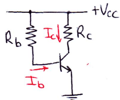
$$\Rightarrow I_b = \frac{I_c}{\beta} = \frac{1}{2\beta} \frac{V_{cc}}{R_c}, \text{ or choose } R_b = \frac{V_{cc} - 0.6V}{I_b} = \frac{1}{2\beta} \frac{V_{cc}}{R_c} \quad (3)$$
