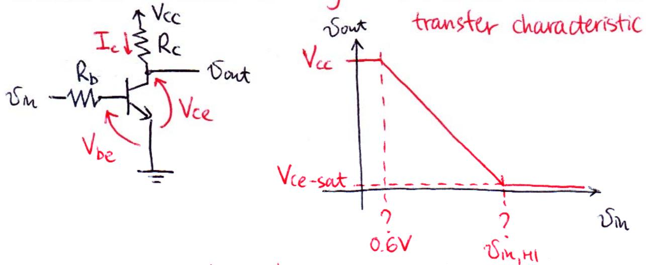
$V_{in,HI}$  : point where transistor goes from active to saturation, i.e.  $\beta \cdot I_b = (I_c)_{\max}$
