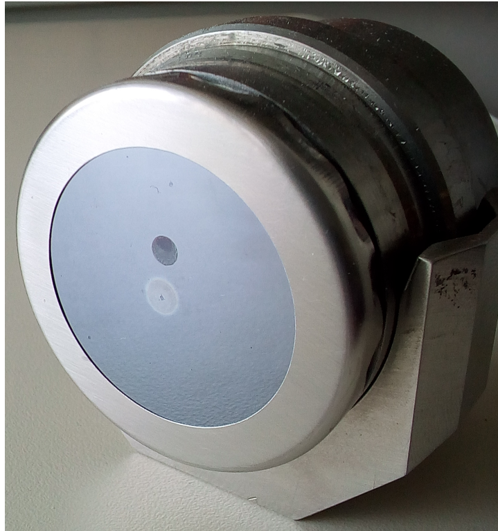
Figure 2.3: A photocathode used in the Cornell photoinjector. The cathode (oxidized, dark gray circle) is placed off center in order to avoid being destroyed by ion back bombardment (center light gray circle) [42].
