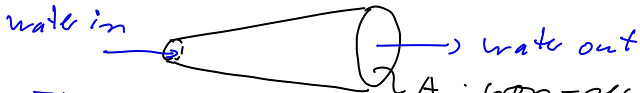
$$\text{Flow rate } F = \frac{dV}{dt} \leftarrow Adx : \text{cross-sectional area}$$
