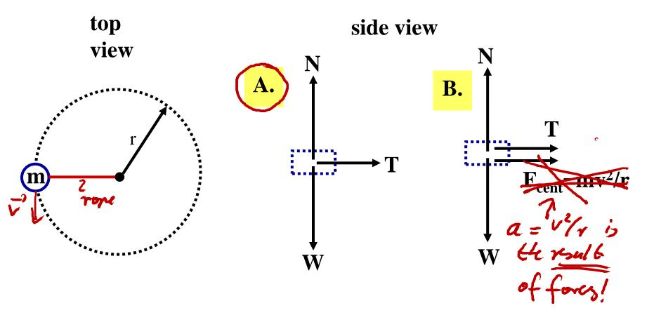
· Z Fon object is cause of a, of circular motion!  $a = \frac{v^2}{r}$  is effect of forms =>  $|\overline{Z}F_{an}a_{j}| = m|\overline{a}| = m\frac{v^{2}}{T}$  if moving in a circle at speed v - no my strious forces ! ( only gravity, forces direct physical contact ) - Never show Z Fonob; = Frat on a FBD! -) never show my as a fore on a FBD for circulay motion!
