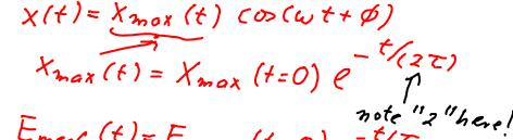
=) Emech (t)= Emech (t=0)e-tit T: energy decay time in each st=T: \( \int \text{Xmax} \) \( \text{Xmax} \)
