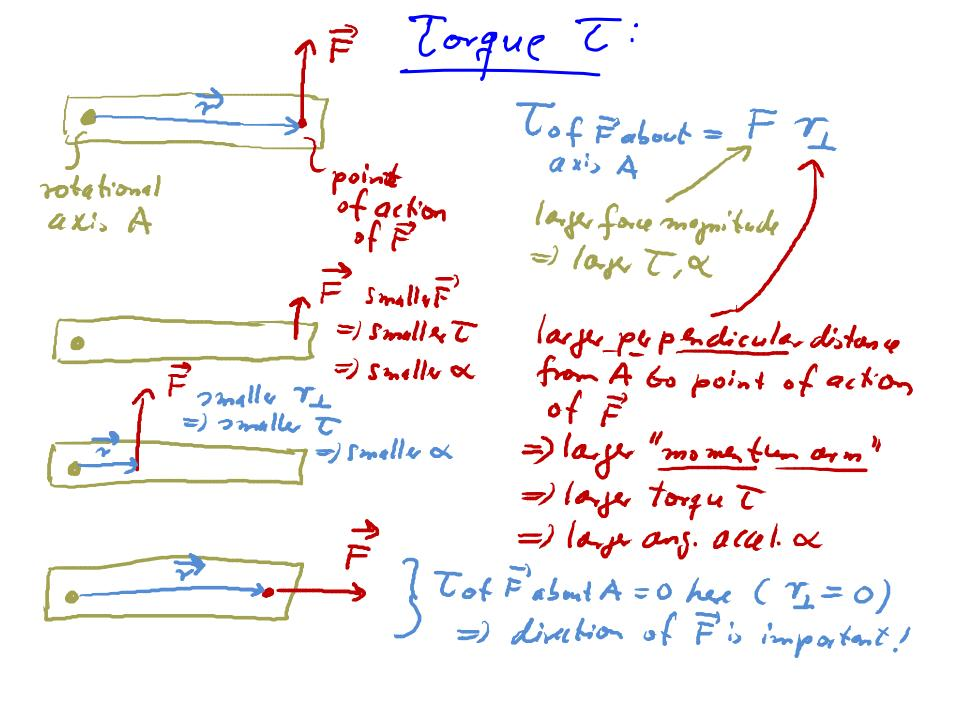
p: angle between Fand ? for F 11 +0 ? : Produce no rotation and no torque about · for FI to ? = T. Sin & Lot E,  $= F_{\perp} \cdot \tau$ (in direction of F, and passing through = + r sin p the point of action) - distance from 11 momentum orm 4 aris A to the line of of Faboutari, A action of force F
