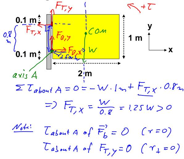
What is the horizontal force exerted on the gate by the top hinge?
