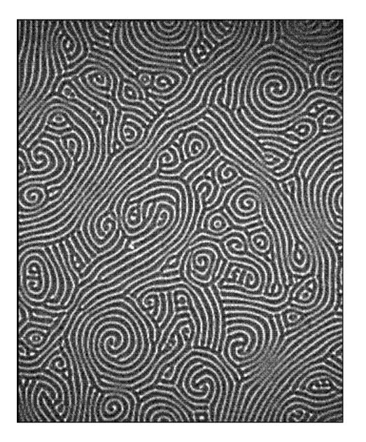
Gas convection between two horizontal glass plates, with heating from below
