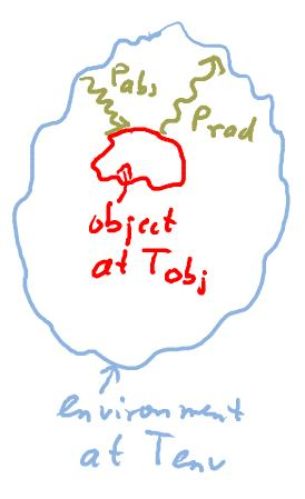
=) Pret radiated = Prad - Pabs = - dQols = (-rate at which from object to environment to environment
