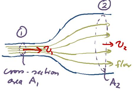
In time of, the volume of fluid enterny at 1 must equal the volume of V2 of fluid leaving at 2 = 0 V2
