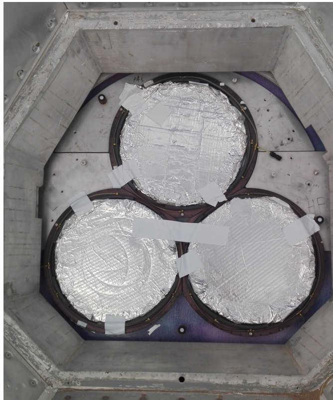
Figure 4.5: Picture showing the Advanced ACTPol camera covered by aluminum foil reflective covers. Picture credit: Rodrigo Quiroga.
