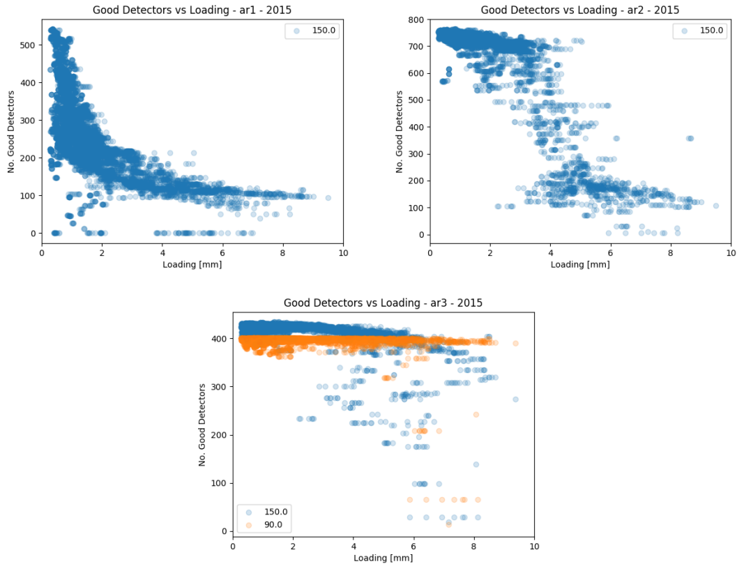
Figure 6.8: Number of detectors which pass the IV-curve cuts vs estimated sky loading, which is given by the PWV / \sin(\text{alt}) for each array in the 2015 observation season. The legends indicate the frequency of the detectors in GHz. Plots contain 26,014 of the 62,359 TODs from the 2015 season.
