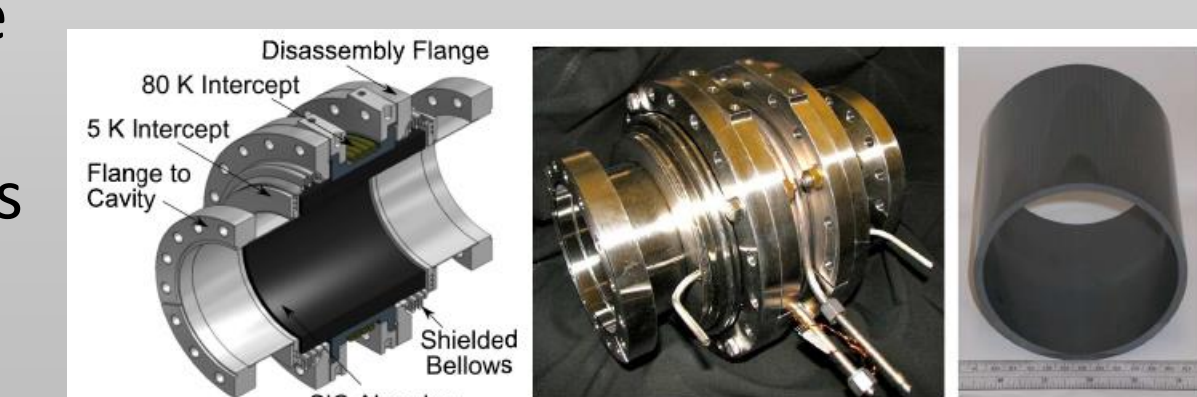
HTC-3 Cross-section, including HOM Loads
